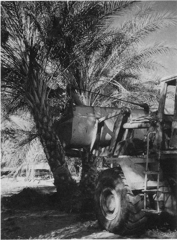
1. A pair of Phoenix dactylifera is hoisted as a single specimen, using a boom on a front-end loader.
