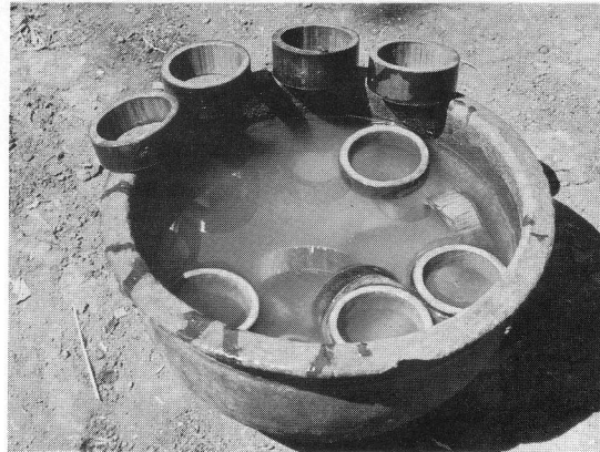
80. Bamboo rings used in molding palm sugar.
